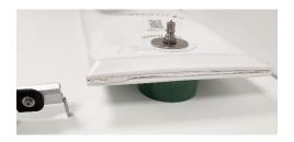
f) Remove the circlip using the pliers provided in the pouch replacement kit.
