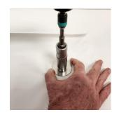
Create a vacuum in the pouch using the passivator provided in the pouch replacement kit connected to the compressor (See passivator usage in the annex)
