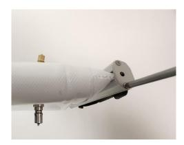
b) Rotate the 2 plates at each end of the high and low fastener.
