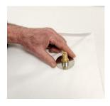
k) Tighten to the specified torque using the torque screwdriver provided in the pouch replacement kit until you hear 2 "clicks".
