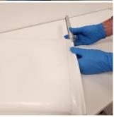
d) Position the Z-folds on the side opposite to this first corner using the spatula, being careful not to damage the pouches or create creases.
